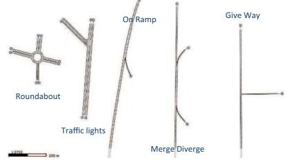
Figure 1. Layout of the five test networks. As the layout changes, the effect of the different parameters on the outputs changes as well.
